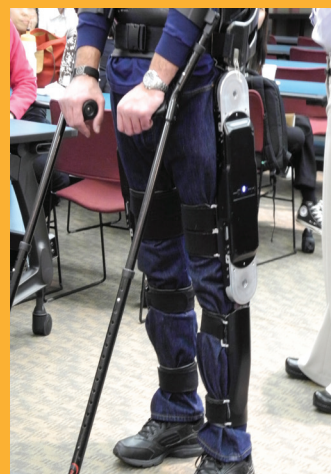
Demonstrating the Indego, Parker-Hannifin's exoskeleton
